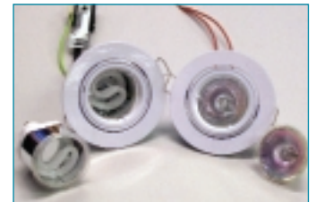
These new 240 Volt compact fluoro down lights, (above left) look just like a halogen down light (right) and fit in the same diameter recess. They offer a lot of advantages in suitable applications.
