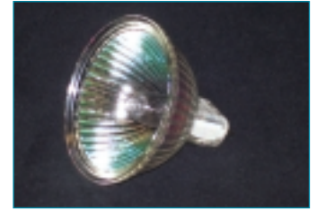
Halogen lamps produce a considerable amount of heat and are suitable mainly for spot lighting, as opposed to general lighting.
